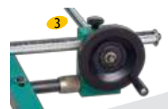
Wheel operated adjustment of the back gauge
